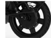
In-house built 3 KW Hub Motor
